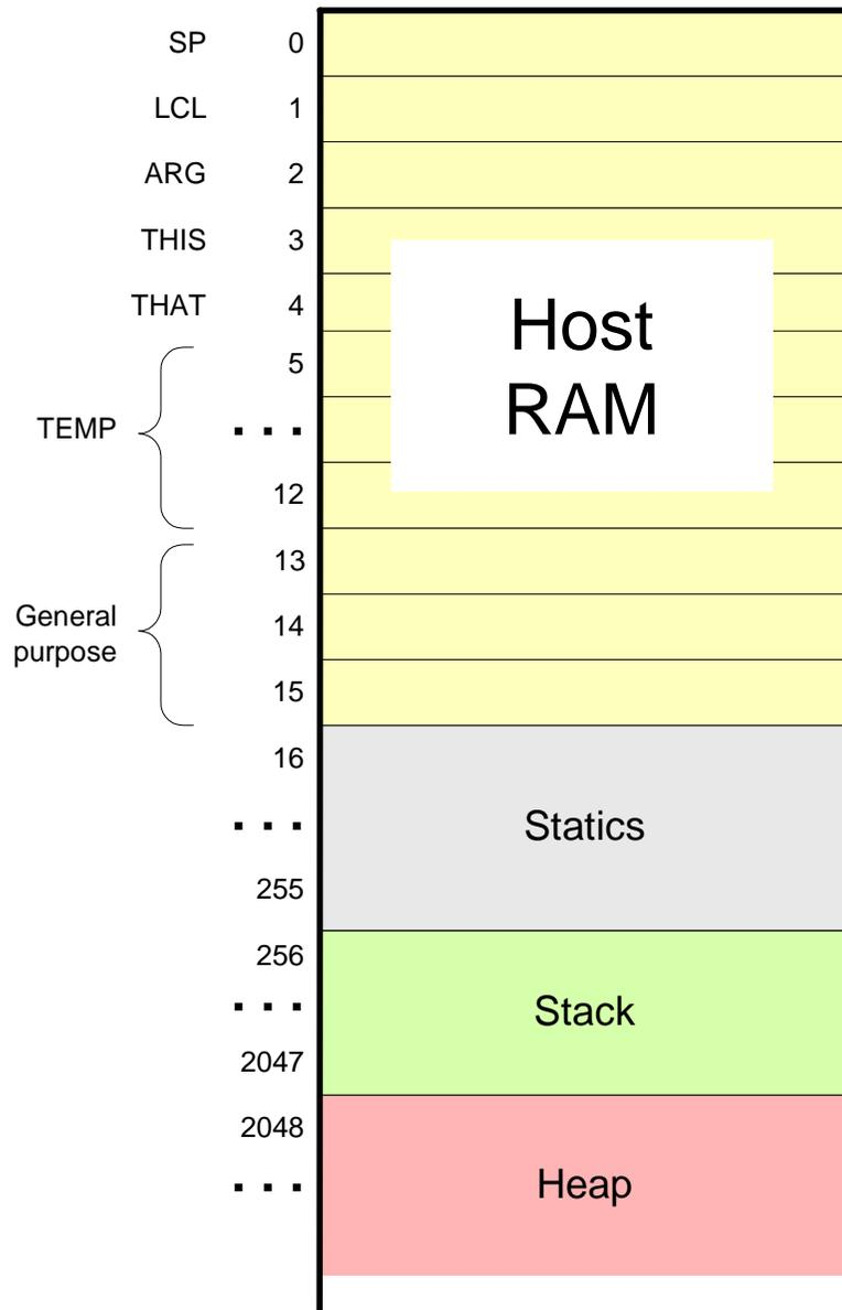
**Basic idea:** the mapping of the stack and the global segments on the RAM is easy (fixed); the mapping of the function-level segments is dynamic, using pointers
