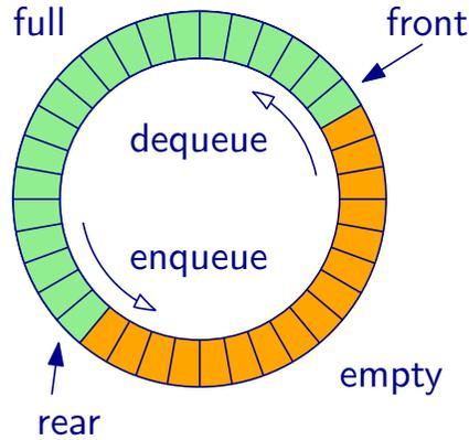
Since we do not have circular memory, we have to simulate that using a linear array, and two index pointers.
